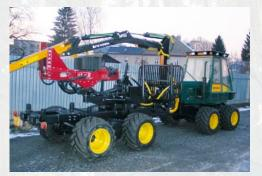
ENTRACON prepare dual harwarders where introduce new efficiency and flexibility to wood harvesting. A single machine can be quick transformed in a few minutes from an efficient harvester into a powerful forwarder, and vice versa.
